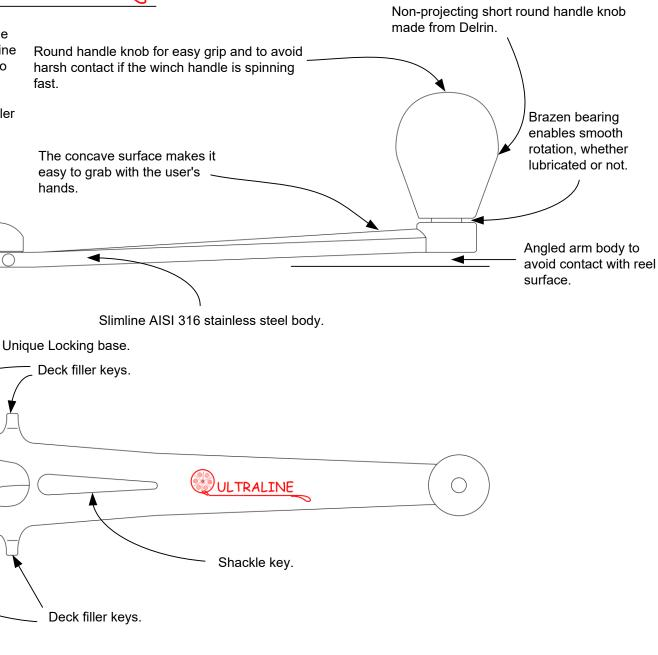
Slimline, thumb lock to lock winch handle in socket profile.
